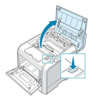
**CAUTION**: If you open the left cover for a few minutes, the imaging unit can be exposed to light. This causes damage to the imaging unit. Close the top and left cover should the setup need to be halted for any reason.
